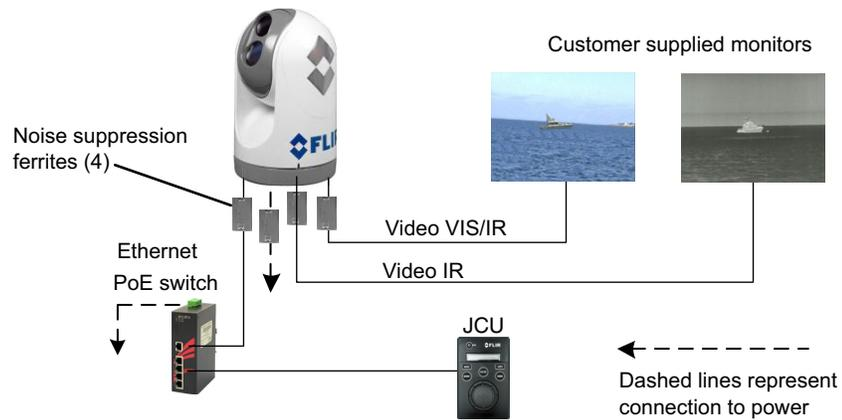
Figure 1-1: Basic installation using a customer PoE switch
