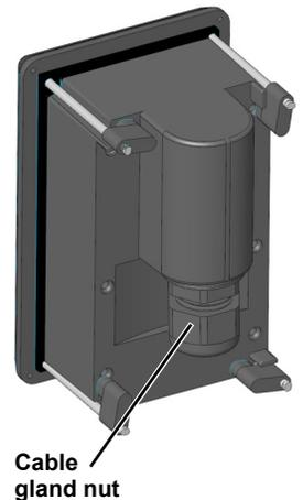
5. Insert the JCU into the hole and secure by turning the 4 corner screws clockwise. Rotate each screw one full turn and ensure the mounting clamps are rotated outward from the JCU housing. Tighten the screws to draw the mounting clamps up against the mounting surface and then tighten another quarter or half turn. Do not overtighten the screws.
